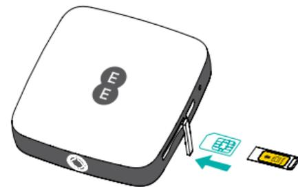
Use the included SIM tool to help fully insert the Nano-SIM until it clicks into place.
