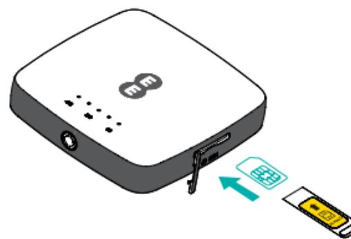
Use the included SIM tool to help fully insert the Nano-SIM until it clicks into place.
